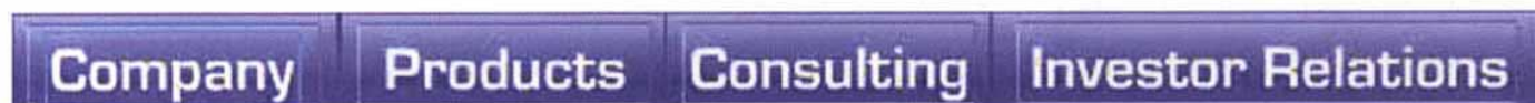
Figure 1: This navigation bar is not optimized for localization, as the text abuts the sides of the buttons leaving no room for text expansion. As a result, the point size of the text will have to be considerably reduced, the buttons widened or the translation abbreviated.
